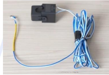
Yellow CT: measure the current on the main AC cable
