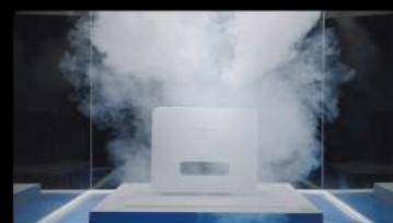
Salt Spray Test
