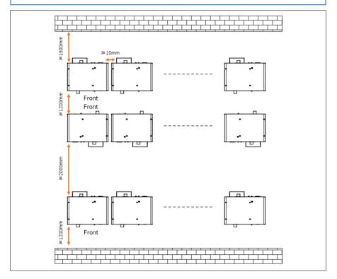
Fig2a. Clearance requirement
