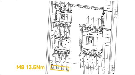
Figure 6. load side - copper busbar terminal connection
