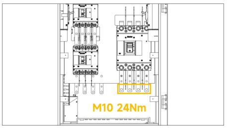
Figure 5. grid side - copper busbar terminal connection
