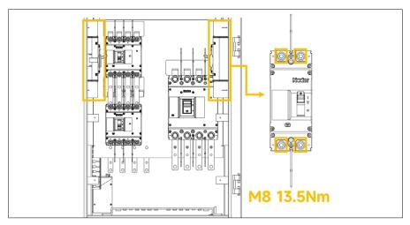
Figure 4. PV side - copper terminal connection
