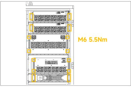
Figure 3. Screw position - module
