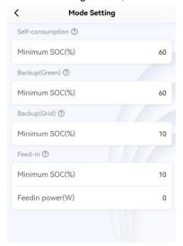
Process 4: Select the Off-grid Working Status Setting, and configure the minimum SOC threshold during the execution of the off-grid mode;
