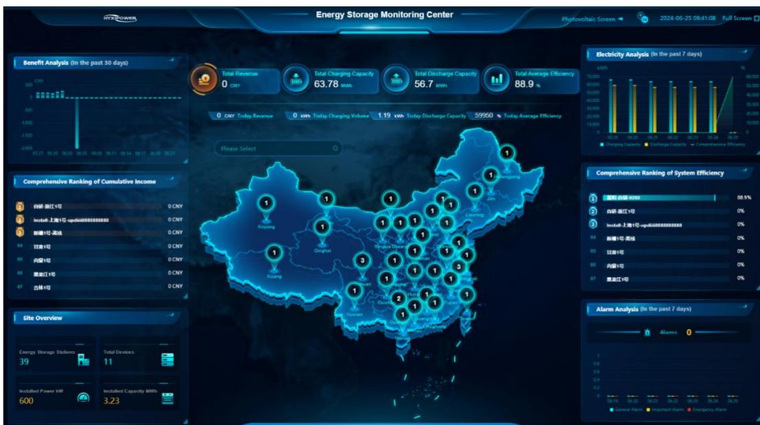
Step 5: The Energy Storage Monitoring Center dashboard displays the distribution of plants on the national map, and by clicking on the plant icon, it displays the plant's Safe Operating Days, Installed Capacity, Installed Power, and Total Charging Capacity and Total Discharging Capacity, etc.
