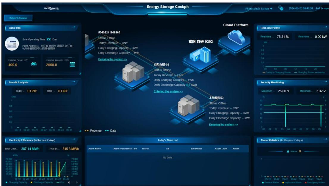
Step 7: The Energy Storage Cockpit displays the online and offline status of the current plant's energy storage device, the Today Revenue, and the Daily Charging Capacity and Daily Discharging Capacity, and the data on both sides display the Basic Info of the energy storage plant, Benefit Analysis, Electricity Efficiency, Real-time Power, Security Monitoring, Alarm Statistics, and Today's Alarm List, etc.
