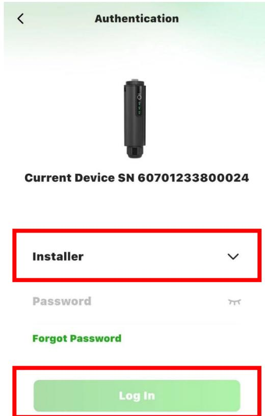
**Step 3** : Device login, initial password: **hyxi0607**. (If the password is incorrect, please try **12345678** ) Log in and change the password, then save. (Record the new password. If you forget the password next time, you can **quickly press the DCS RESET button 4 times to restore the factory settings**)
